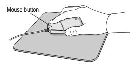
If the arrow doesn't move, make sure that the cables connecting the mouse and keyboard are secure and that your mouse is positioned as shown in the illustration.
